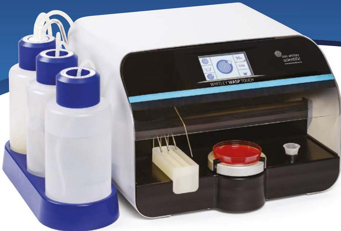
**Whitley WASP Touch** is a totally new spiral plater designed for contemporary microbiology laboratories. Equipped with our new automated intelligent monitoring software which guides you through set up and daily check routines, prompts cleaning fluid replenishment, when to empty the waste container and a host of other unique user benefits. Simple to use, it provides real cost savings and process improvements, at a very affordable price.
