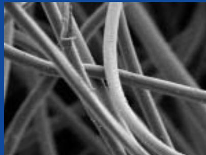
**Figure 2.** A non-inoculated Aquacel Ag dressing (10k x magnification)
